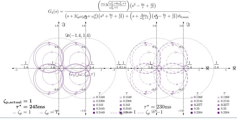
SUFFICIENT FREQUENCY DOMAIN CRITERION CAN BE CHECKED GRAPHICALLY FOR LOWER ORDER SYSTEMS  $\rightarrow$  DELAY MARGIN CAN BE DERIVED USING NYQUIST PLOT & CIRCLE CRITERION AS  $\bar{\tau}^{\star} = \min_{\zeta_{p}} (\max (\{\tau \mid G_{1}(j\omega, \zeta_{p}, \tau) \in \mathfrak{D}(-\vartheta_{1,\max}, \vartheta_{1,\max})\}))$
