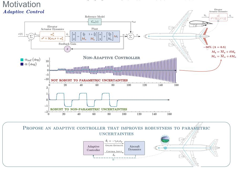
$\frac{Z_q}{V_0} \sim \frac{Z_{\delta_e}}{V_0} \sim \frac{Z_{\delta_e}}{V_0} \sim 0, \ M_\alpha = -\omega_p^2, \ M_q = -2\zeta_p\omega_p, \ M_{\delta_e} = 1, \ (\zeta_p, \omega_p, k_p) = (-1, 1, 1), \ (\zeta_\eta, \omega_\eta, k_\eta) = (0.89, 17, 17^2), \ (\zeta_m, \omega_m, k_m) = (1, 3, 1)$
